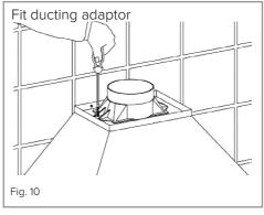
IMPORTANT SAFETY WARNING: ONLY USE THE SCREWS PROVIDED WITH THE EXTRACTOR TO MOUNT THE DUCTING ADAPTOR. THE USE OF LONGER SCREWS MAY CAUSE DAMAGE TO THE INTERNAL WIRING WHICH WILL NOT BE COVERED BY THE WARRANTY.
