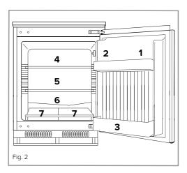
The fridge shelves can be moved according to the storage requirements within the fridge section. To move the shelf, lift up the front section and then pull it outwards. To replace, slide the shelf back into the slot, and lower the front section.
