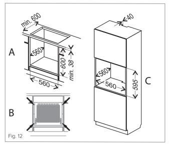
holes. Remember the housing should not be free-standing but be secured to the wall and/or adjacent fittings.
